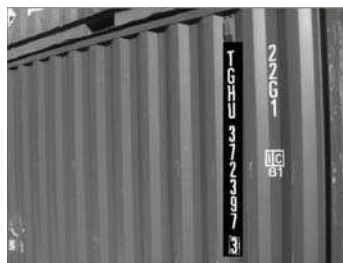
Fig. 3. Binarization result of vertically-arranged identifier areas
