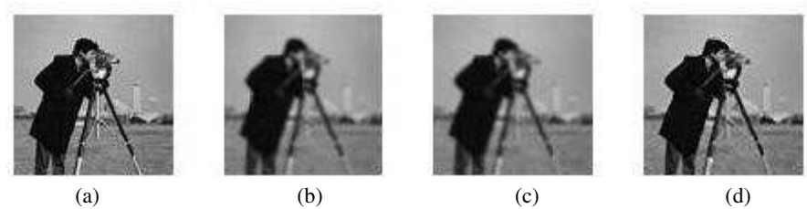
Fig. 4. Cameraman images (a) original cameraman image; (b) burred image; (c) restored image with Wiener Filter (d) restored image using proposed method
