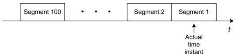
Fig. 3. The division of the EEG waveform into 100 segments
