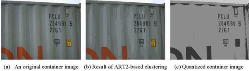
Fig. 1. An original container image and the processed results
